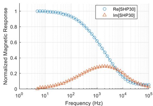
Fig. 5. Normalized real and imaginary magnetic response of the SHP30 sample. The solid lines show the reconstructed response from the hydrodynamic size distribution.
