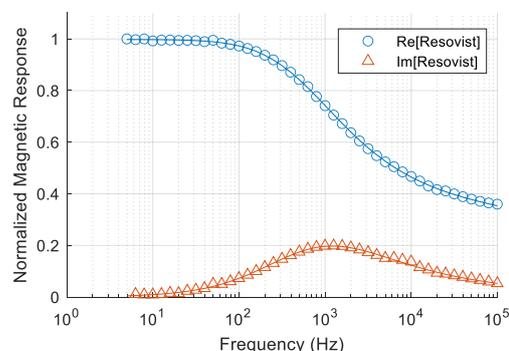
Fig. 4. Normalized real and imaginary magnetic response of the Resovist sample. The solid lines show the reconstructed response from the hydrodynamic size distribution.
