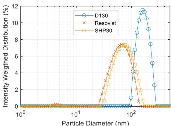
Fig. 2. Hydrodynamic sizes of MNP samples determined using the dynamic light scattering (DLS) method.
