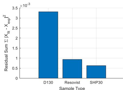
Fig. 7. Residual sum of the reconstructed AC magnetic responses for the D130, Resovist, and SHP30 samples.
