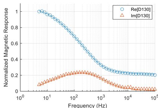
Fig. 3. Normalized real and imaginary magnetic response of the D130 sample. The solid lines show the reconstructed response from the hydrodynamic size distribution.
