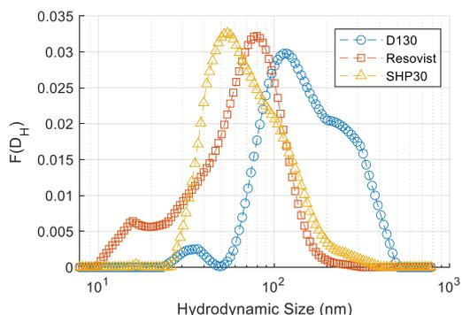
Fig. 6. Hydrodynamic size distributions of the D130, Resovist, and SHP30 samples.
