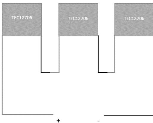
Figure 9: Illustration Connection TEG in Flat Arrangement
