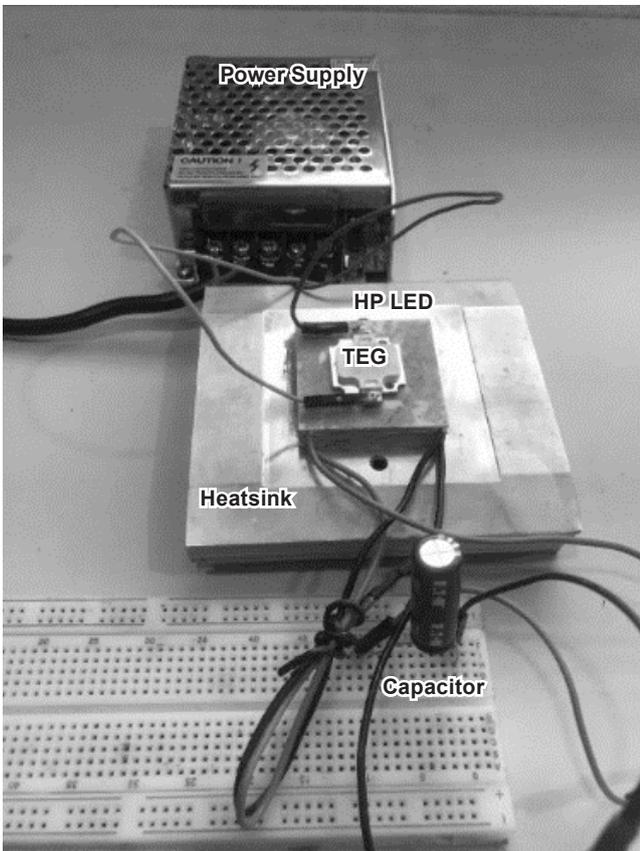
Figure 4: TEG Output Connected with Capacitors for Energy Storage
