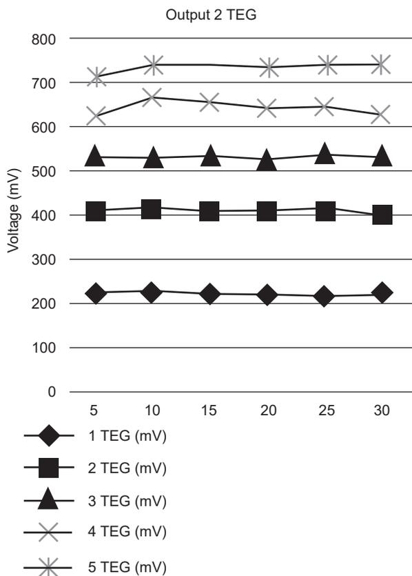
Figure 8: Graph Shows Increase in TEG Output with Total TEG
