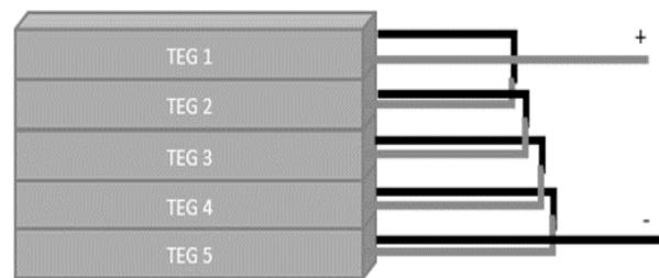
Figure 7: Illustration Connection of TEG in Cascade Arrangement
