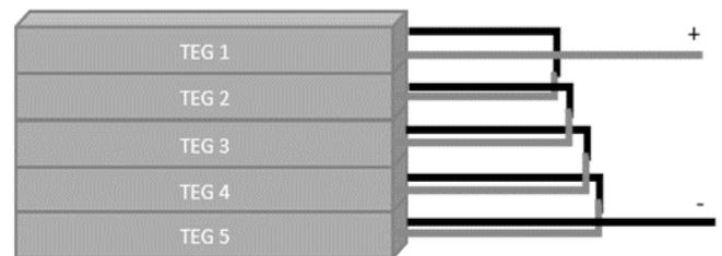
Figure 2: Illustration Connection TEG in Series
