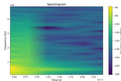
Fig. 16: Spectral characteristics of the recorded signal in the case of an interaction voltage of 5kV
