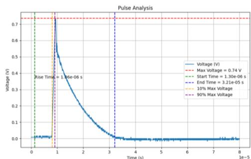
Fig. 7. Characteristics of the recorded signal in the case of an interaction voltage of 5kV
