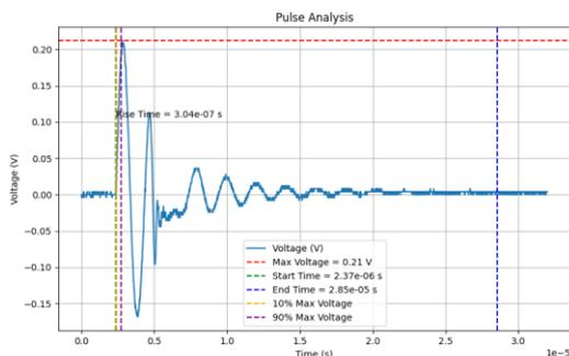
Fig. 8. Characteristics of the recorded signal in the case of an interaction voltage of 5kV
