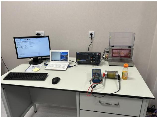
Fig. 1. View of the control panel with measurement instrumentation and PEF interaction chamber.
