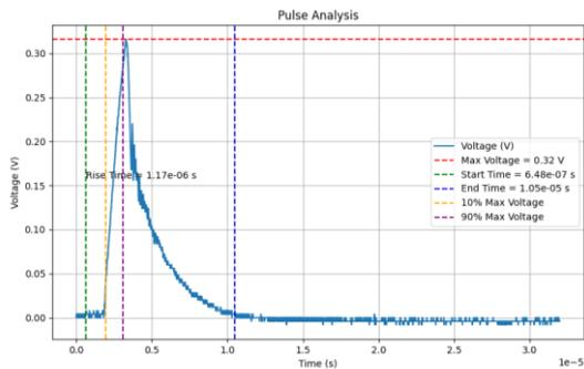
Fig. 6. Characteristics of the recorded signal in the case of 5kV interaction voltage
