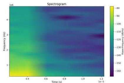
Fig. 13. Spectral characteristics of the recorded signal in the case of 5kV interaction voltage.
