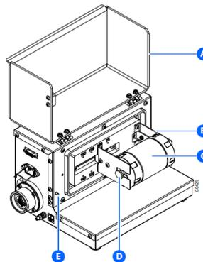
Fig. 3. Diagram of the PEF impact chamber: A) Cover - Safety feature. Must always be closed during operation; B) Holder – Holder for the jar. Serves as connector for the electrodes; C) Screw – For securing the jar in the holder. Can be moved between jars; D) D- Momentary switch- Safety feature. The PEF chamber cannot be operated with the momentary switch in extended position
