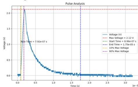
Fig. 10. Characteristics of the recorded signal in the case of an interaction voltage of 50kV
