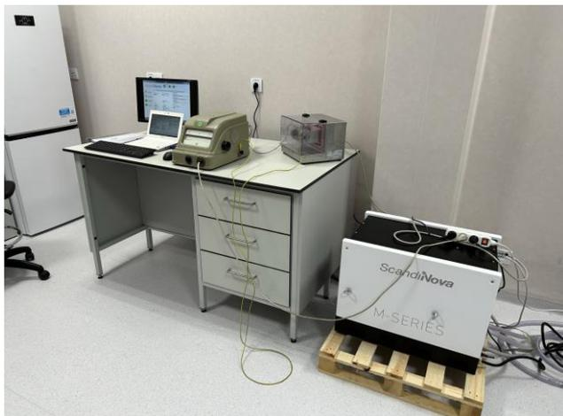
Fig. 2. View of the ScandiNova M100 test stand with a generator unit for PEF generation.
