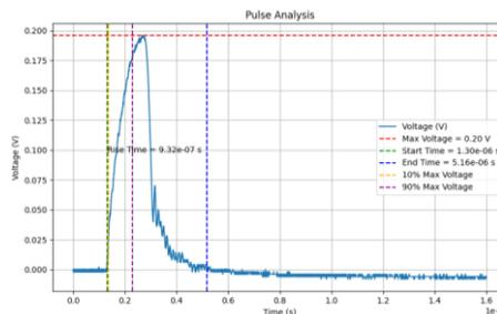
Fig. 5: Characteristics of the recorded signal in the case of an interaction voltage of 5kV
