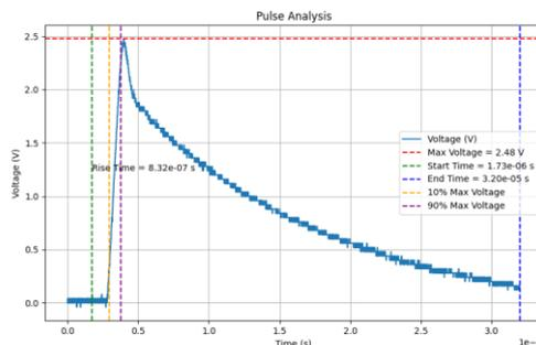
Fig. 11. Characteristics of the recorded signal in the case of an interaction voltage of 5kV
