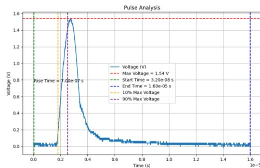
Fig. 9. Characteristics of the recorded signal in the case of an interaction voltage of 50kV
