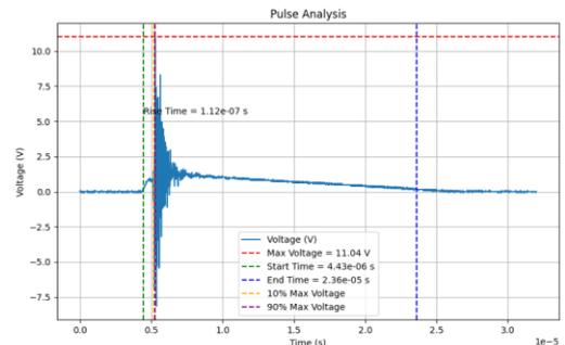
Fig. 12. Characteristics of the recorded signal in the case of an interaction voltage of 50kV
