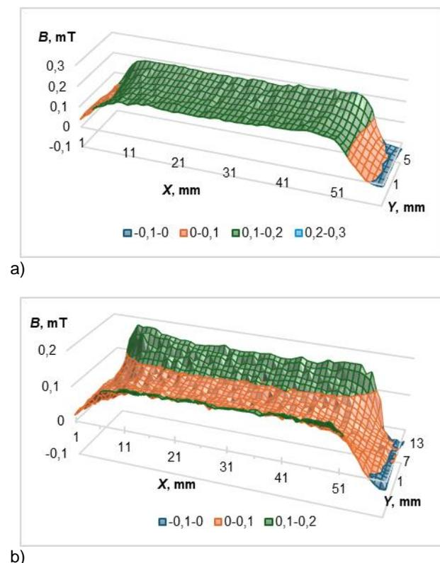
Fig. 3. 3D map of the distribution of magnetic flux density for  $I=200$  mA and distance between coils: a) 20 mm, b) 40 mm
