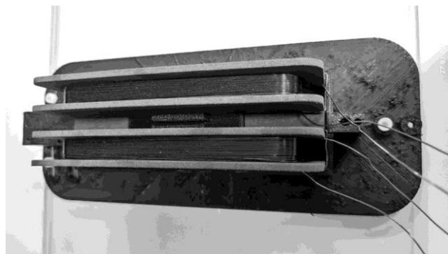
Fig. 2. 3D printed polyamide coil formers for windings, created using the SLS method
