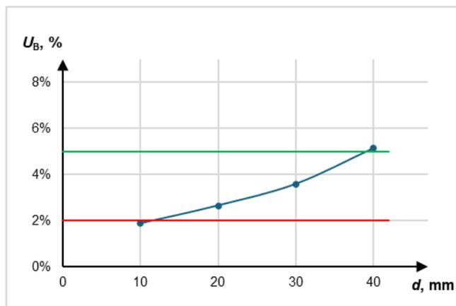
Fig. 4. Magnetic field uniformity for  $I=200$  mA
