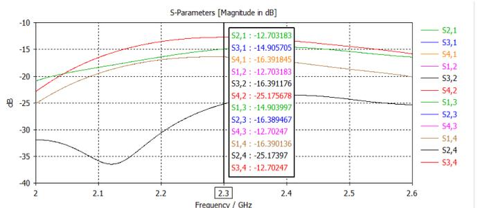
Fig. 5. Simulated S parameters for isolation between antennas.
