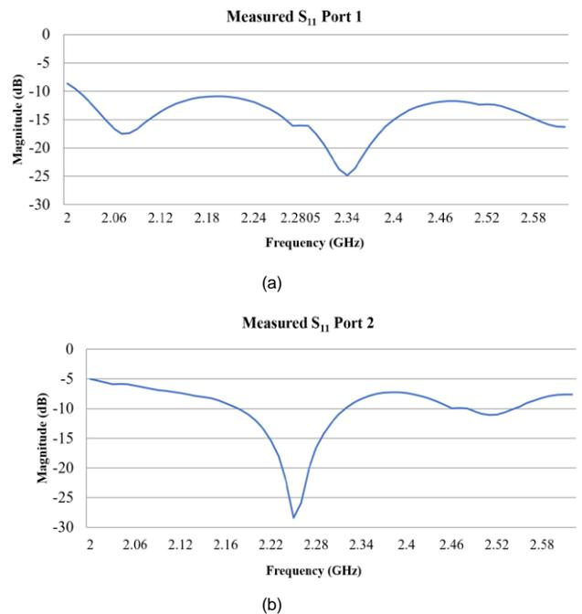
Fig. 6. Measured  $S_{11}$  of (a) antenna 1 (port 1) and (b) antenna 2 (port 2).
