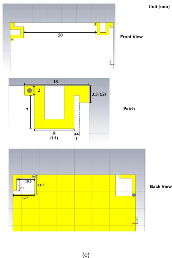
Fig. 1. Geometry of the 4-Antenna Array for MIMO Operation in the 5G Mobile Operation (a) Overall Front View (b) Overall Back View (c) Detailed Design
