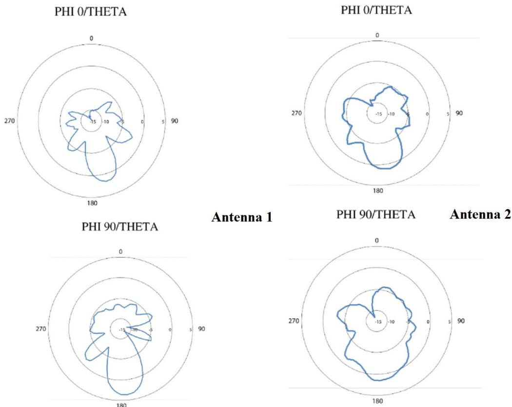
Fig. 7. Measured two-dimensional radiation pattern.
