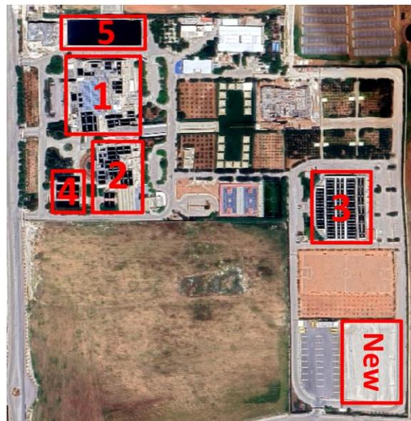
Fig. 1: Top satellite view of MEU campus showing the main five locations where the solar modules are mounted. The "new" box represents the proposed new PV system location.
