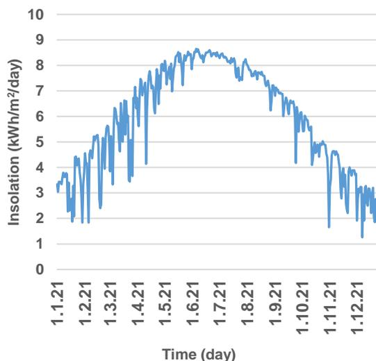
Fig. 9: Hourly satellite solar insolation for the new PV system location.
