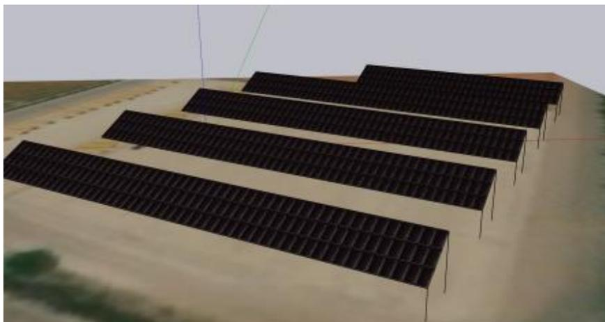
Fig. 7: 3D model of the new PV system arrays
