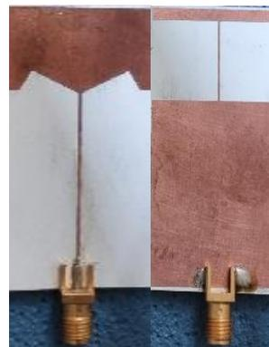
Fig. 3. Optimized view of the physical antenna model - front and back.
