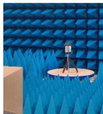
Fig. 4. Appearance of the laboratory stand during the measurements of radiation patterns of the antenna.
