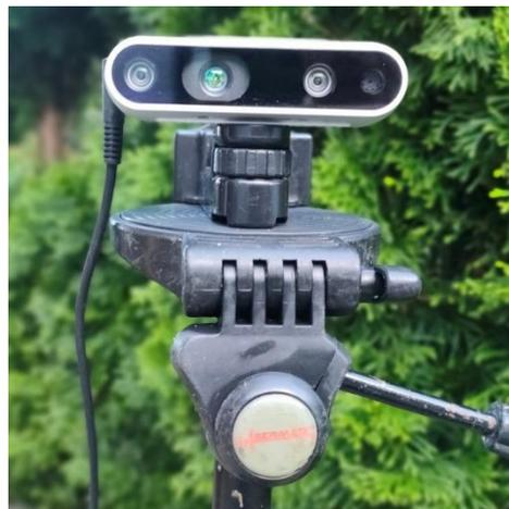
Fig. 2. Mounting the stereo camera on a tripod to prevent position changes during tests
