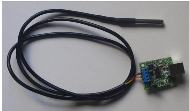
Fig. 14. DS18B20 thermometer and 1-wire to USB converter module; the data from the thermometer can be read directly in an application written in C/C++ programming language.
