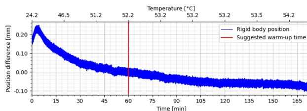
Fig. 10. Measurement drift in the  $x$  axis; the data has been normalised and shows the difference in measurement compared to the position when the system was fully warmed up (60 minutes).
