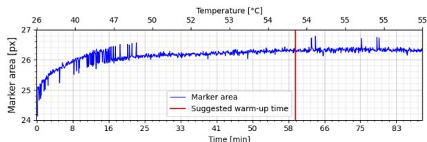
Fig. 7. The changes in the marker area during the test. The temperature of the camera affects the area and could limit the visibility of the marker if it is too low. The diameter of the marker used was 12.7 mm.
