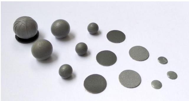
Fig. 1. Comparison of different passive markers. The differences are in the material used, diameter and type (spherical, flat).
