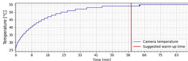
Fig. 6. The rate of the temperature rise when tracking space is captured.
