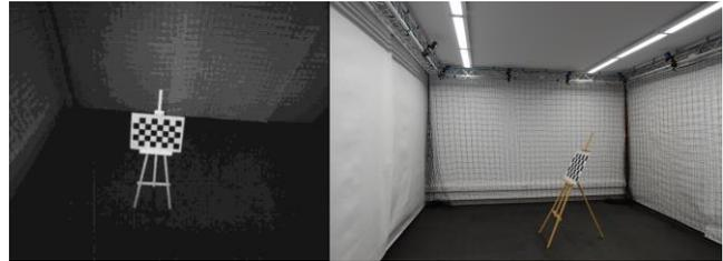
Fig. 2. Camera placement process. For the best setting of the camera orientation, the real-time camera preview and the positioning tool were used (here improper camera's orientation is visible). The brightness and contrast of the left part of the image were changed for better visibility.
