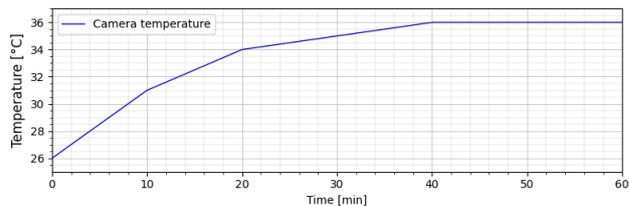
Fig. 5. The change of temperature in the time when the system is only powered on and capturing is not active. Due to the very slow temperature rise, the number of measurements was limited for readability.
