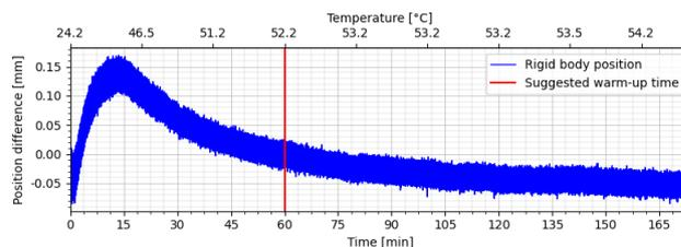
Fig. 11. Measurement drift in the  $y$  axis; the data has been normalised and shows the difference in measurement compared to the position when the system was fully warmed up (60 minutes).
