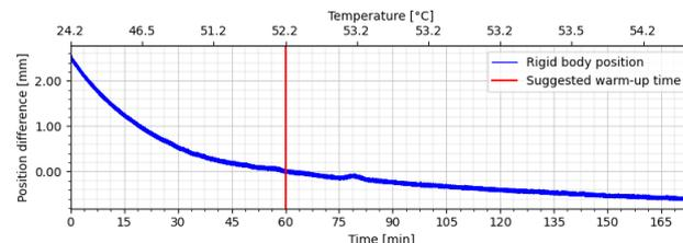
Fig. 12. Measurement drift in the  $z$  axis; the data has been normalised and shows the difference in measurement compared to the position when the system was fully warmed up (60 minutes).
