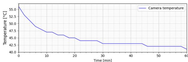
Fig. 8. The change of temperature in the time when the system is powered on and capturing is not active.
