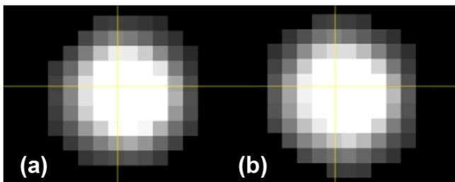
Fig. 4. Comparison of marker area depending on the camera temperature; the marker diameter was 12.7 mm; the (a) shows the marker area at temperature of 32°C; the (b) shows the marker area at temperature of 54°C.
