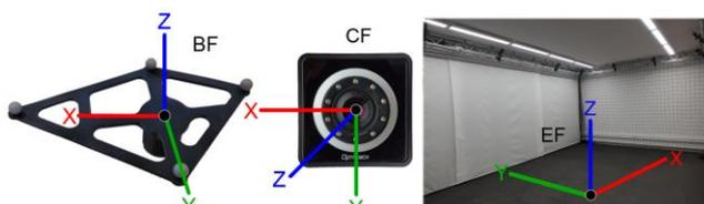
Fig. 9. Comparison of coordinate systems. The EF means Earth Frame and it is related to global OptiTrack coordinate system. The BF means Body Frame and it is related to tracked object (tool). The CF means Camera Frame and it is related to single camera.
