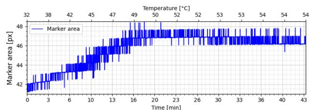
Fig. 3. Example of correlation between marker size and temperature; the diameter of the marker used was 12.7 mm.
