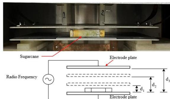
Fig. 1 : A radio frequency (RF) heating setup designed.
