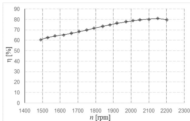
Fig.2. The efficiency characteristic for  $\text{SmC}_{20}$  magnet material
