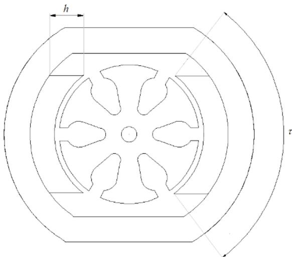
Fig.1. Structure of the brushed DC motor
