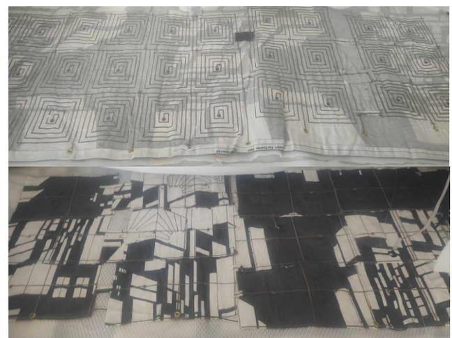
Fig. 5. Prototype of the heating mat in actual dimensions of 200 x 90 cm. Top layer - heating elements, bottom layer - connections and power lines.
