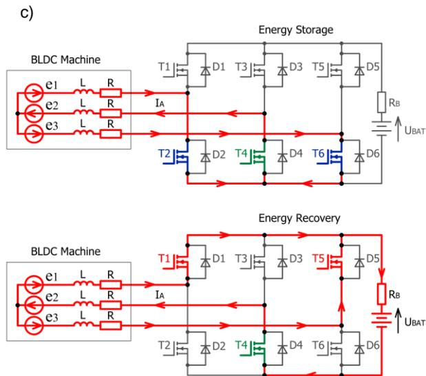
Fig. 2. New regenerative braking control method: a) switching signals and back EMF voltages, b) switching sequence and Hall sensor signals, c) current flow path in the system during energy storage and recovery stages
