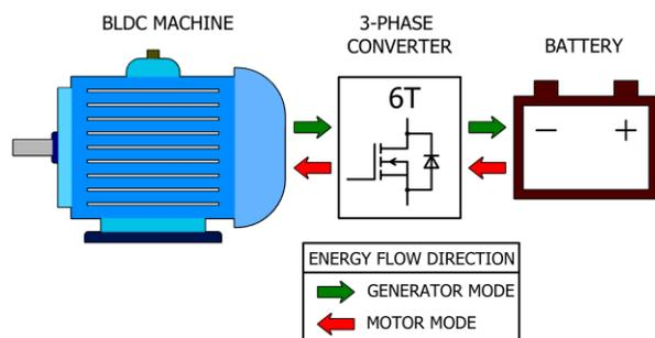
Fig. 1. The classic BLDC machine drive system
