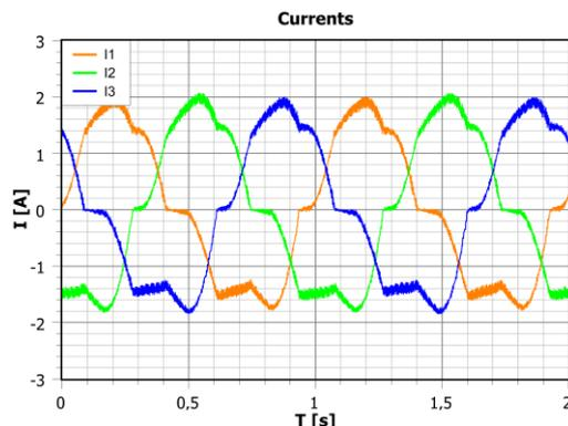
Fig. 9. Waveforms of phase currents of the machine
