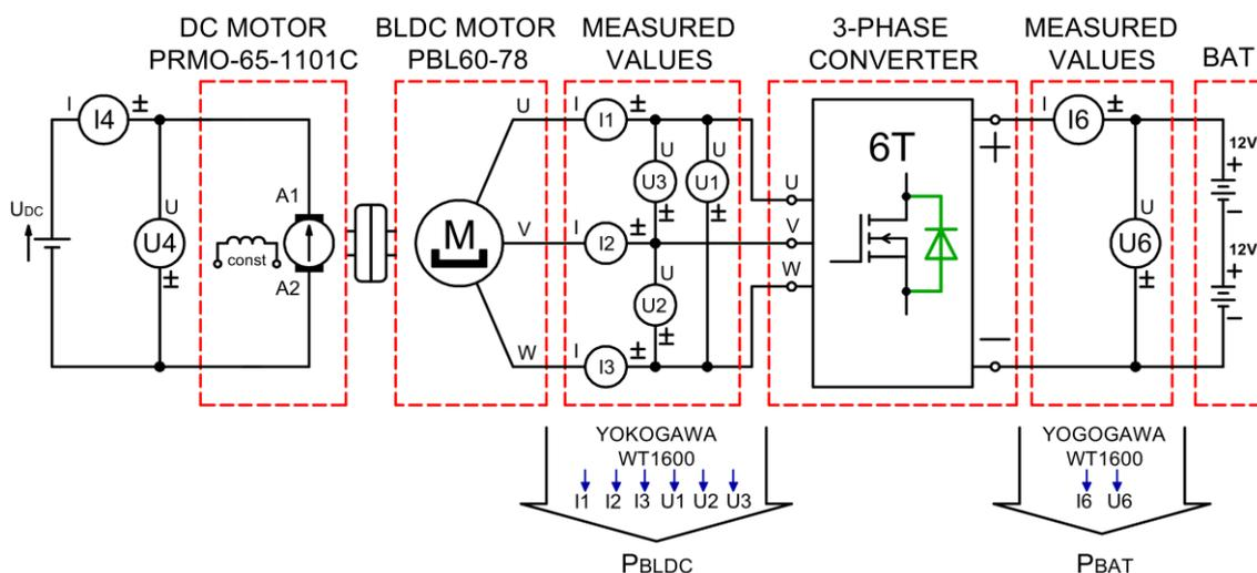
Fig. 7. Diagram of the measurement system
