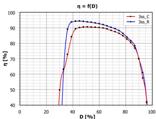
Fig. 10. Converter efficiency as a function of the PWM duty cycle at maximum power returned to the battery
