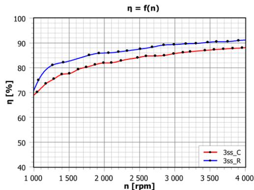
Fig. 11. Converter efficiency as a function of the rotational speed of the BLDC machine at maximum power returned to the battery
