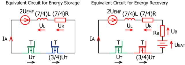
Fig.4. Resultant circuits for the energy storage and recovery stages
