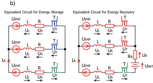
Fig. 3. Equivalent circuits for: a) conduction of two phases of the BLDC machine, b) conduction of three phases of the BLDC machine
