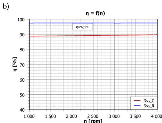
Fig. 5. Converter efficiency as a function of: a) the PWM duty cycle, b) the rotational speed of the BLDC machine at maximum power returned to the battery
