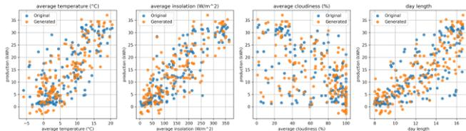
Fig. 7. Scatter plots for the first model comparing real data and data generated from the posterior model separately for each factor affecting the amount of energy produced from solar panels. The values of both types are consistent, especially in terms of data distribution, which is the most important aspect. Compared to priors, the charts also show values that deviate more from the distribution, known as outliers.
