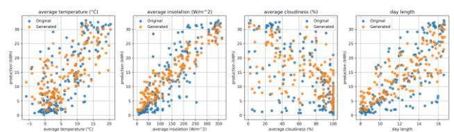
Fig. 10. Scatter plots for the second model comparing real data and data generated from the prior model separately for each factor affecting the amount of energy produced from solar panels. The values of both types are consistent, especially in terms of data distribution, which is the most important aspect.
