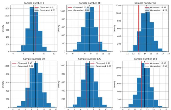
Fig. 23. Histograms for the experimental model showing the distribution of energy consumption for one day in every month along with overlaid real and analysis-generated values. These values generally overlap.
