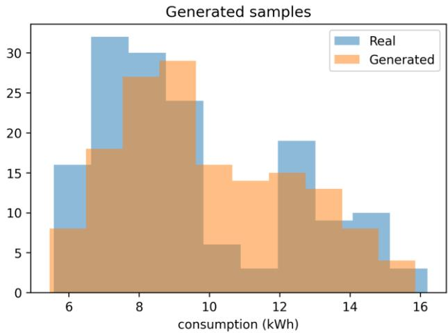
Fig. 14. Chart for the experimental model comparing histograms of real data and data generated from the prior model for energy consumption. The model shows quite a high degree of consistency, and the histograms are similar; however, the bimodal structure of the actual data is not particularly visible.
