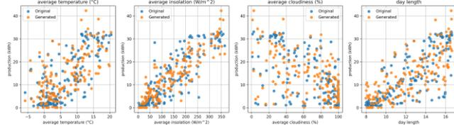
Fig. 12. Scatter plots for the second model comparing real data and data generated from the posterior model separately for each factor affecting the amount of energy produced from solar panels. The values of both types are consistent, especially in terms of data distribution, which is the most important aspect. Compared to priors, the charts also show values that deviate more from the distribution, known as outliers.
