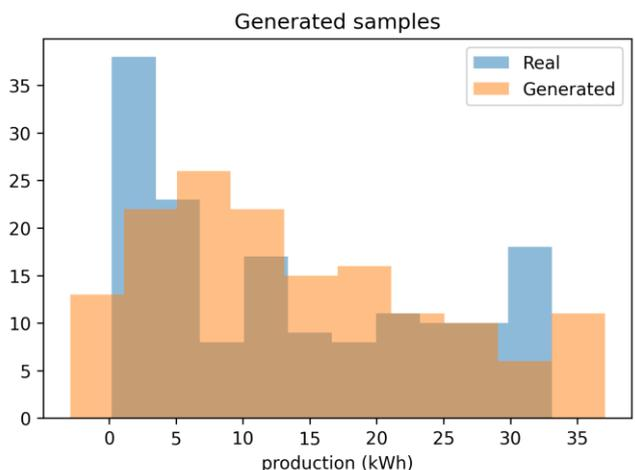
Fig. 6. Chart for the first model comparing histograms of real data and data generated from the posterior model for energy production. In terms of achieved values, the model is quite consistent; however, the distribution of generated data slightly differs from the irregular, hard-to-replicate distribution of real-world data.
