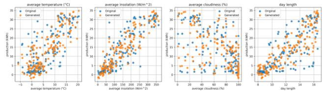
Fig. 5. Scatter plots for the first model comparing real data and data generated from the prior model separately for each factor affecting the amount of energy produced from solar panels. The values of both types are consistent, especially in terms of data distribution, which is the most important aspect.
