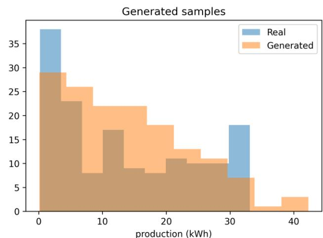
Fig. 11. Chart for the second model comparing histograms of real data and data generated from the posterior model for energy production. The range of achieved values generated is larger (due to maximum values) than in the case of real-world data.
