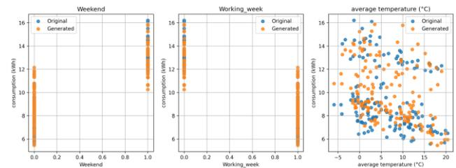
Fig. 15. Scatter plots for the experimental model comparing real data and data generated from the prior model separately for each factor affecting the amount of energy consumed. The values of both types are consistent, especially in terms of data distribution, which is the most important aspect.
