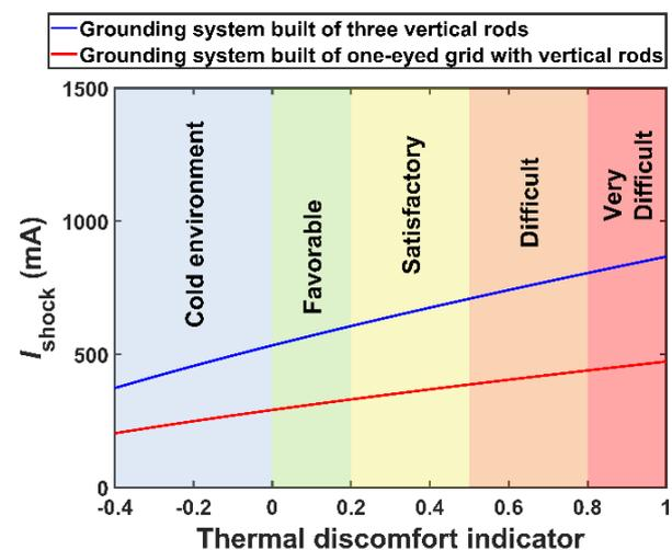
Fig. 3 Calculated values of the shock current for the considered earthing structures and hand-to-hand shock path.
