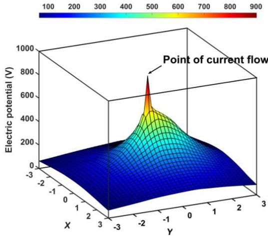
Fig. 1. Distribution of electric potential on the ground surface for an earthing electrode composed of three vertical rods 1.5 m long.
