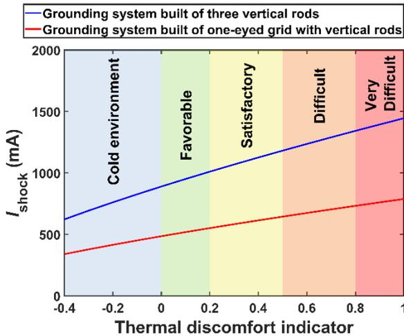
Fig. 4. Calculated values of the shock current for the considered earthing structures and the hand-foot shock path.
