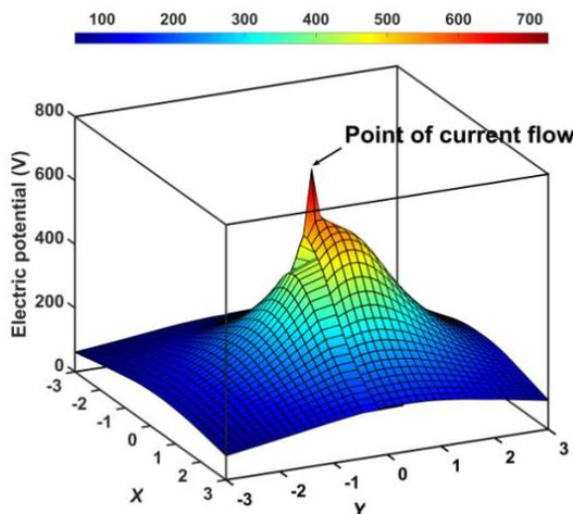
Fig. 2. Distribution of electric potential on the ground surface for a grid earthing with vertical rods 1.5 m long
