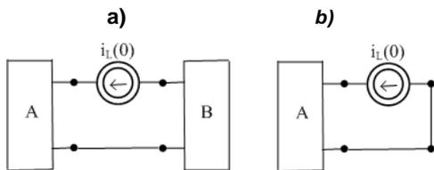
Fig. 2. Two 1-ports connection through current source. A) 1-port B is present, b) 1-port B is omitted.
