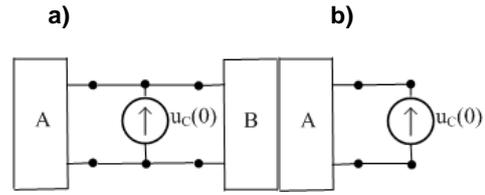
Fig. 3. Two 1-ports connection with parallel voltage source. a) 1-port B is present, b) 1-port B is omitted.
