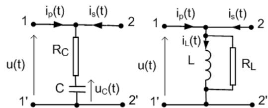
Fig. 5. Recognized 2-port. a) capacitive circuit, b) inductive circuit
