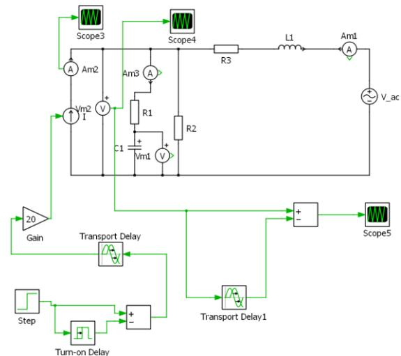
Fig. 7. PLECS block diagram for the grid with capacitive port
