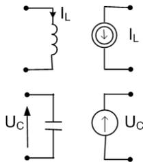
Fig. 1. Substitution of the inductor current and the capacitor voltage.
