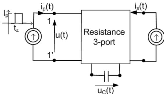
Fig. 6. Resistance 3-port with one capacitive port
