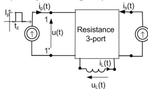
Fig. 12. Resistance 3-port with one inductive port
