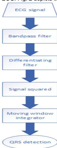
Fig. 2 The cascade of the filtering process of the ECG leading to QRS complex detection.
