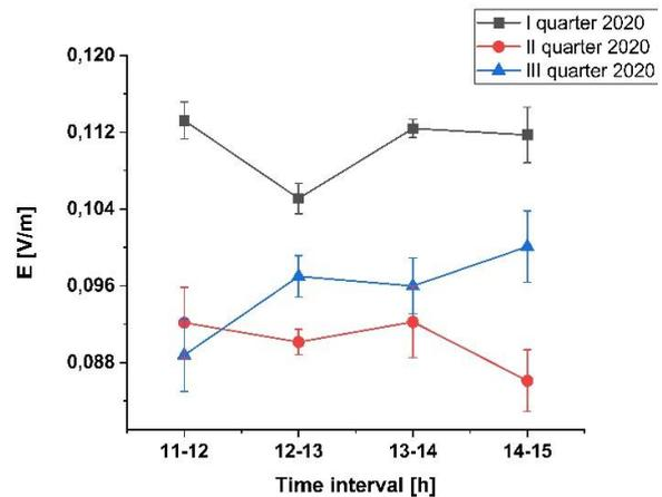
Fig. 1. Changes in total electromagnetic field strength (for all analyzed frequency bands) from 11 a.m. to 3 p.m. averaged for the first three quarters of 2020.
