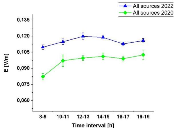
Fig. 2. Daily changes in the intensity of the radiofrequency component of the electromagnetic field measured at the described location. The results show the field strength from all emitting sources in the analyzed frequency range.
