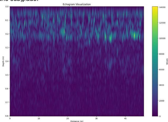
Fig.6. Signal envelope section for selected road
