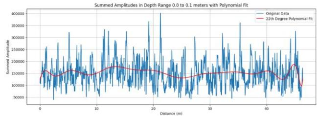
Fig.6. Summed GPR signal amplitudes in the depth range from 0 m to 0.1m
