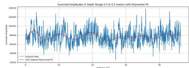
Fig.8. Summed GPR signal amplitudes in the depth range from 0.3m to 0.5m
