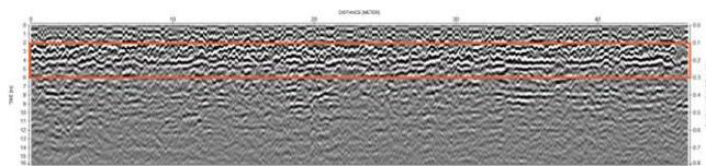
Fig.4. GPR image of a concrete road with the analyzed range from 0.1 m to 0.3 m marked
