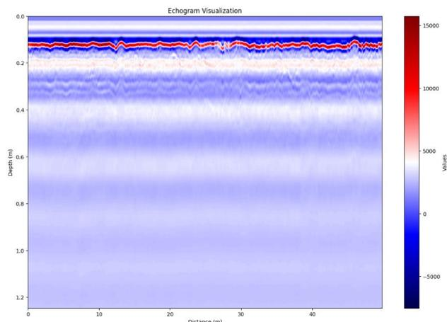
Fig.2. Example of raw GPR data
