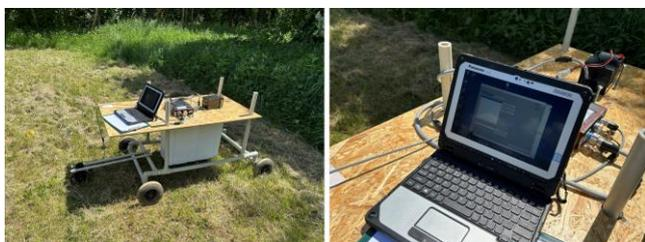
Fig.1. View of the GPR measuring system and the measuring software interface
