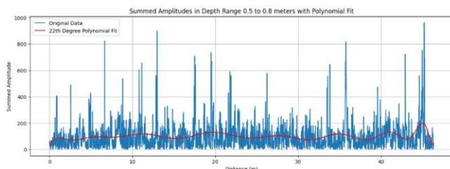
Fig.9. Summed GPR signal amplitudes in the depth range from 0.5m to 0.8m
