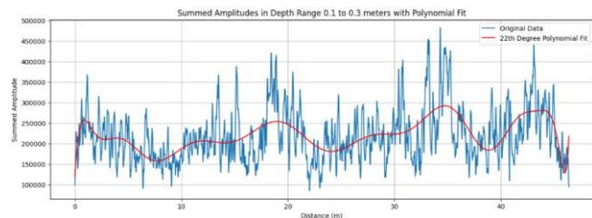
Fig.7. Summed GPR signal amplitudes in the depth range from 0.1m to 0.3m
