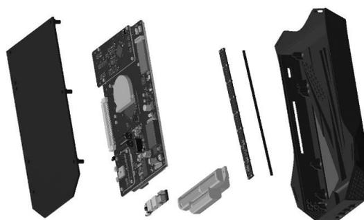
Fig. 1. UST-EIT dual tomograph for bladder monitoring backpack construction
