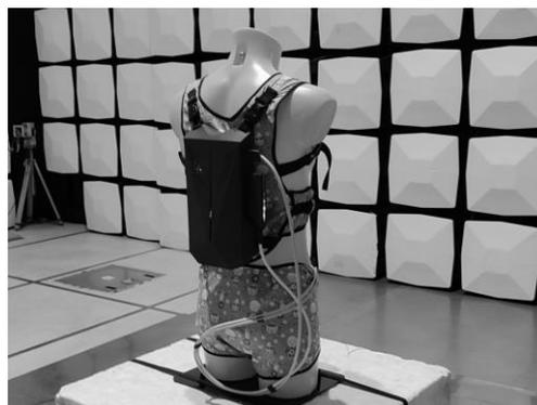
Fig. 4. UST-EIT tomograph for monitoring the lower urinary tract mounted on a phantom during radiated immunity and radiated emissions tests in the frequency range 30 MHz – 1 GHz.
