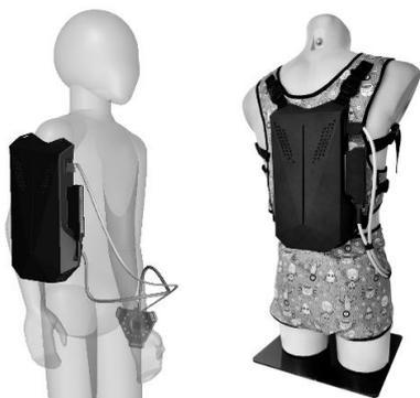
Fig. 2. UST-EIT dual tomograph for bladder monitoring mounted on a phantom.
