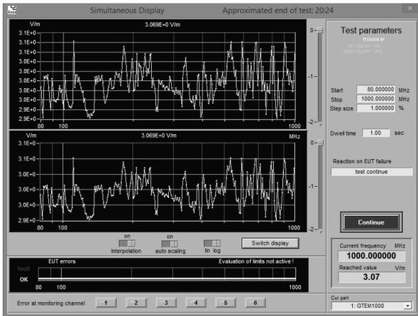
Fig. 7. Radiated Immunity Test – 3V/m
