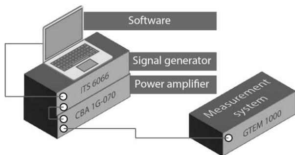
Fig. 4. The functional block diagram of Radiated Immunity Test
