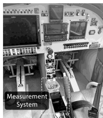
Fig. 1. Installation of the measurement system during a test flight: Aero AT-3
