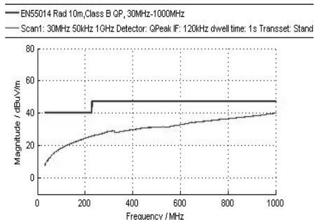
Fig. 6. Measurement of radiated emission of the measurement system with reference to the limit values (PN-EN55014)
