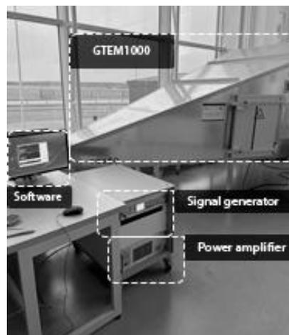
Fig. 5. Set of Radiated Immunity Test
