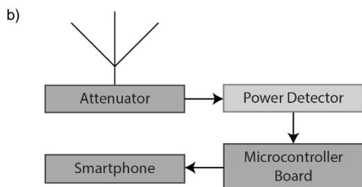
Fig. 2. The proposed measurement system to measure the electric field: a) a picture of the measurement system; b) its block diagram
