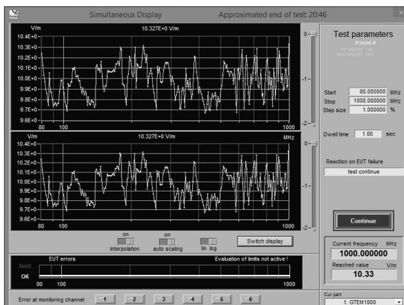
Fig. 8. Radiated Immunity Test – 10 V/m
