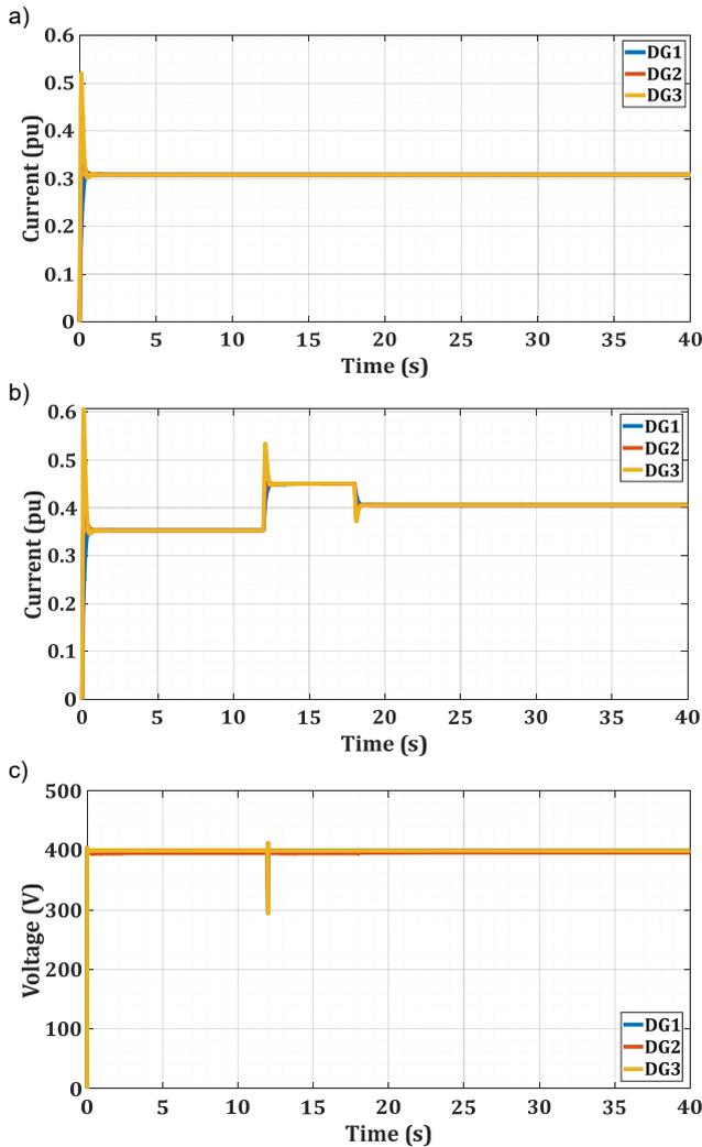
Fig. 8. Power sharing test of the proposed current sharing method. (a) Supplied current by DGs in pu. (b) Supplied current by DGs in pu considering load variations. (c) Microgrid's voltage.
