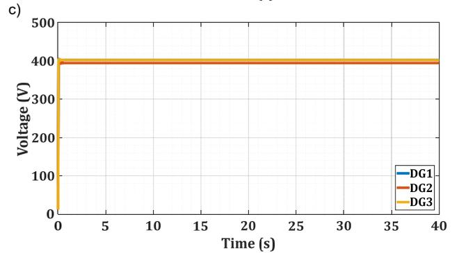
Fig. 6. Power sharing test of the power sharing method in [26]. (a) Active power in pu. (b) Reactive power in pu. (c) Microgrid's voltage
