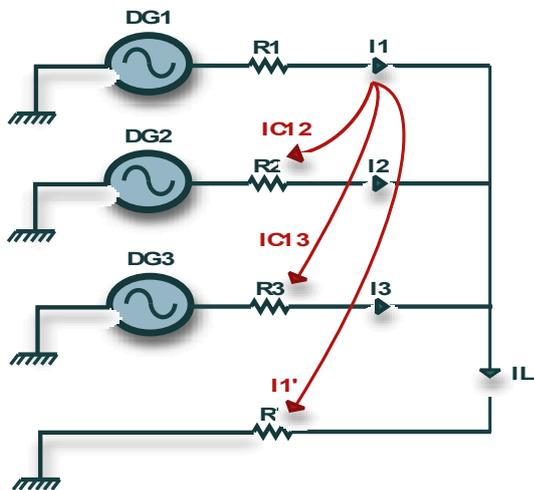
Fig. 2. Equivalent circuit of AC islanded microgrid with 3 DGs
