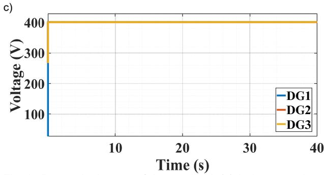
Fig. 4. Power sharing test of droop control. (a) Active power in pu. (b) Reactive power in pu. (c) Microgrid's voltage.
