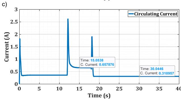
Fig. 5. Circulating current test of droop control. (a) Same transmission lines' impedance value. (b) Different transmission lines' impedance values. (c) Different transmission lines' impedance values with consideration of load variations
