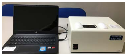
Fig.2. CLE-80 (a minimally invasive cutaneous cholesterol ester level measuring device from Photoscience Co., Ltd.)
