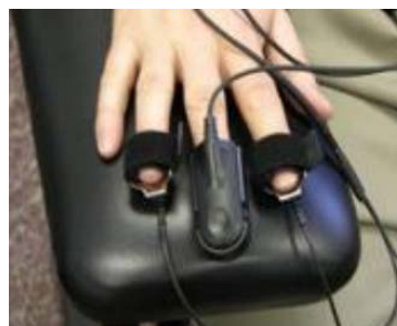
Fig. 5. EDA electrodes placement [15]
