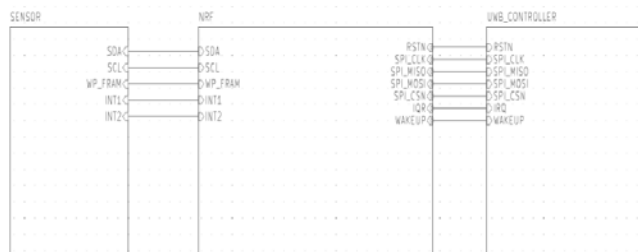
Fig. 1. General wiring diagram of the UWB marker
