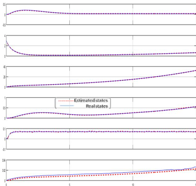
Fig.6 States of the bioreactor controlled by the high order sliding mode controller and supertwist observer with state perturbation
