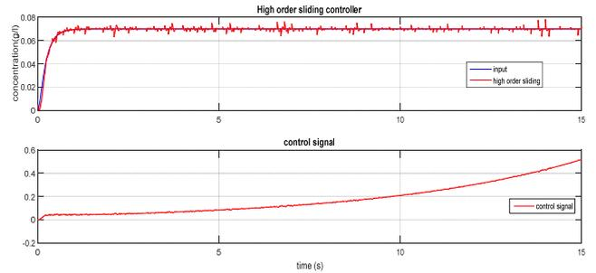
Figure 3 response of the bioreactor controlled by the high order sliding mode controller and supertwist observer with state perturbation
