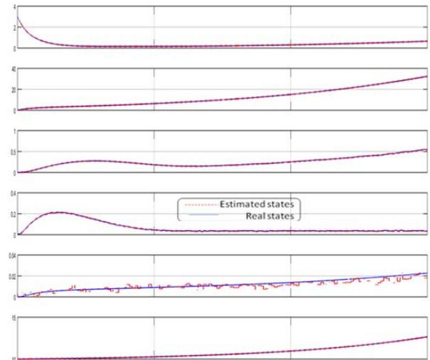
Figure 5 States of the bioreactor for the classic sliding mode controller and sliding observer with state perturbation
