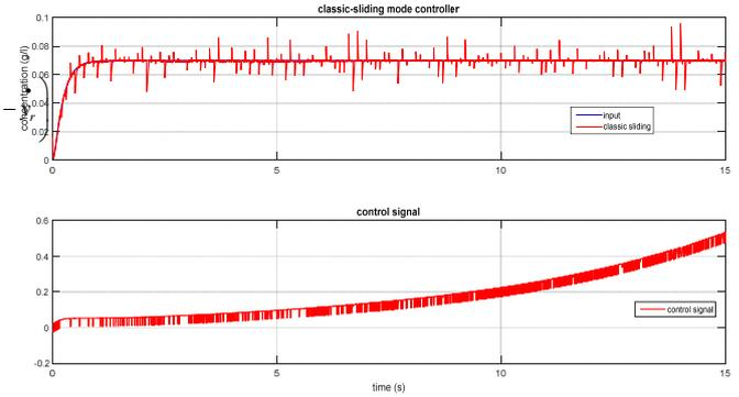
Figure 4 response of the bioreactor for the classic sliding mode controller and sliding observer with state perturbation
