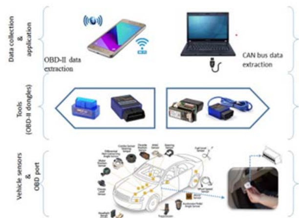
Fig.1. In-Vehicle (telematics) data acquisition through OBD-II interface [3]
