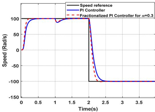
Fig.5. Performance comparison of Fractionalized Order PI controller (for  $\alpha = 0.3$ ) and Integer Order PI controllers for speed tracking at 100 Rad/s.
