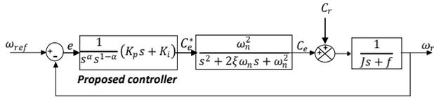
Fig.2. Proposed fractionalized speed control block diagram.
