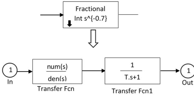
Fig.3. SIMULINK Block Using the Oustaloup Approximation
