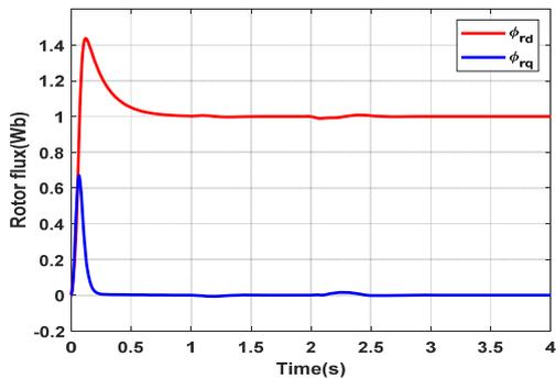
c) Rotor fluxes on the d and q axes.
