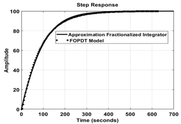
Fig.4. Step response used to obtain the FPDT model.
