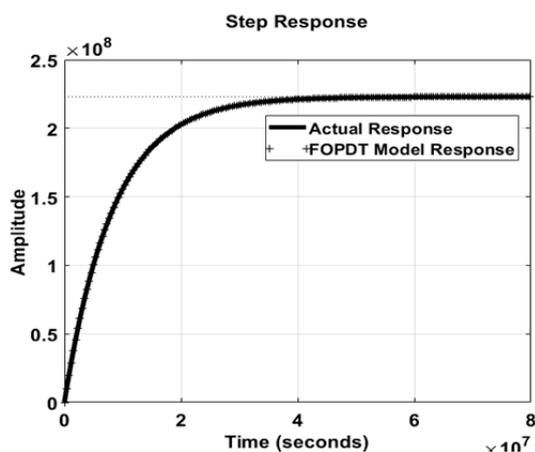
Fig.1. Step response used to obtain the FOPDT model.
