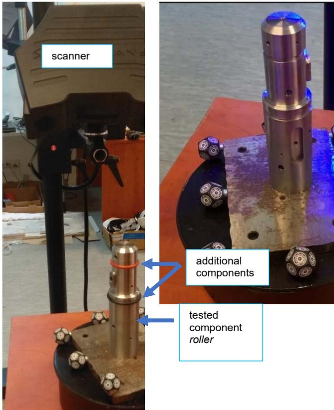
Fig. 9. Scanning the roller
