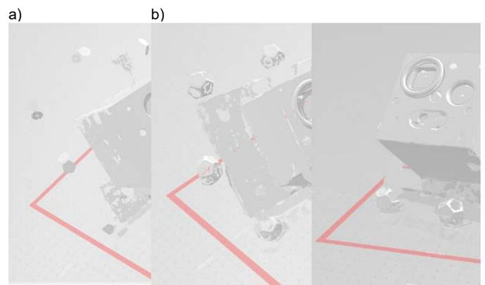
Fig. 8. Scanning results of the cube a) scan result without markers b) scan result of the cube with markers and additional normals
