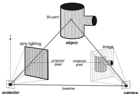
Fig. 1. Structured light scanning method
