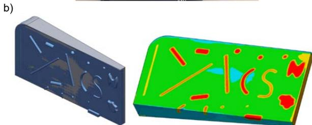
Fig. 4. Testing with blue structured light (a) test stand (b) selected test results
