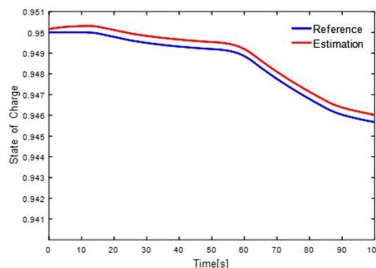
Fig. 7. State of charge battery estimation
