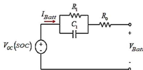
Fig.1. Diagram of cell battery model
