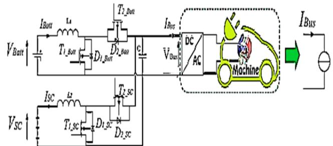
Fig.3. Fully active topological structure of HSS [17]
