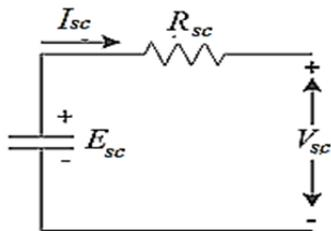
Fig.2. Diagram of cell super capacitor model
