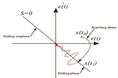
Fig.5. Principle of sliding mode control [28]
