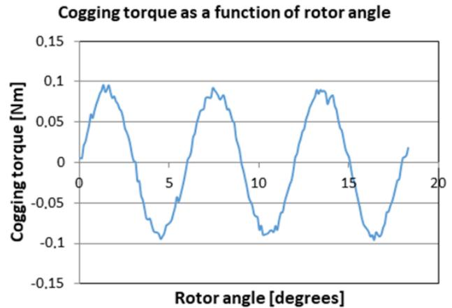
Fig. 9. Computed torque curve
