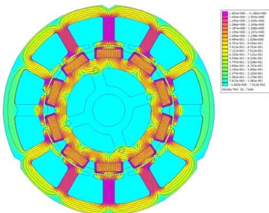
Fig. 3. Magnetic flux distribution in the magnetic circuit of the machine
