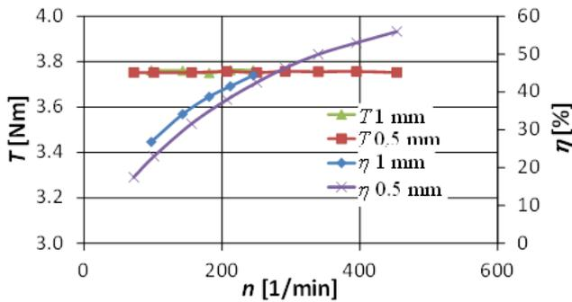
Fig. 6. Mechanical and efficiency characteristics of the developed motors at constant torque ( $T = const$ )
