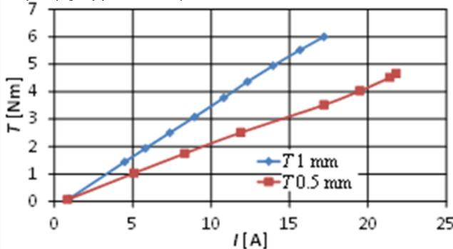
Fig. 8. Dependence of the generated torque on the current for the controller setting  $n = n_{max}$
