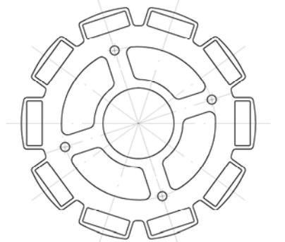
Fig. 2. Shape of the rotor sheets of the developed motor
