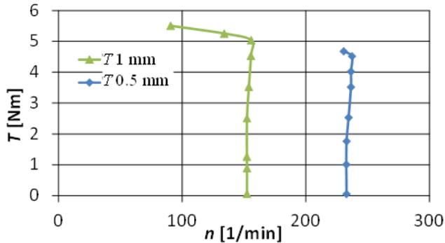
Fig. 7. Mechanical characteristics of the developed motors for the controller setting  $n = 0.5n_{max}$
