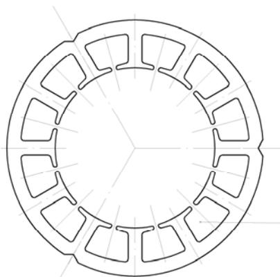
Fig. 1. Shape of the stator sheets of the developed motor
