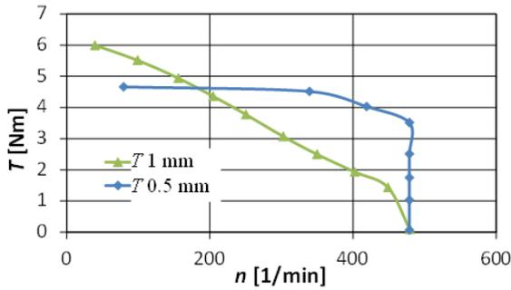
Fig. 5. Mechanical characteristics of the developed motors for the controller setting  $n = n_{max}$
