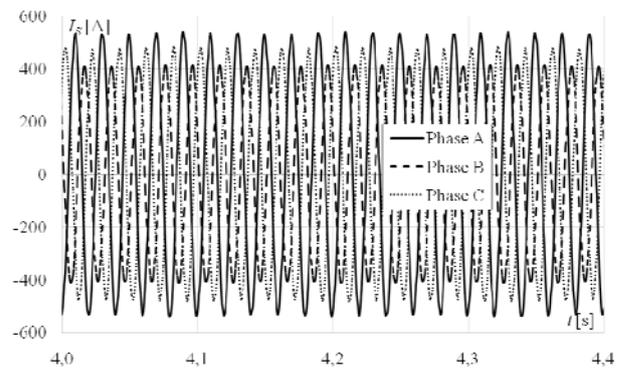
Fig. 7. Waveform of stator current during rated load with coil short-circuit
