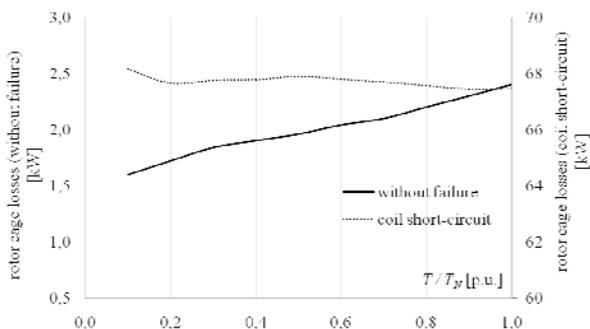
Fig. 11. Rotor cage losses in function of load
