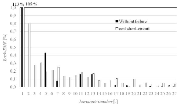
Fig. 4. Back-EMF harmonic distribution between phases A and B
