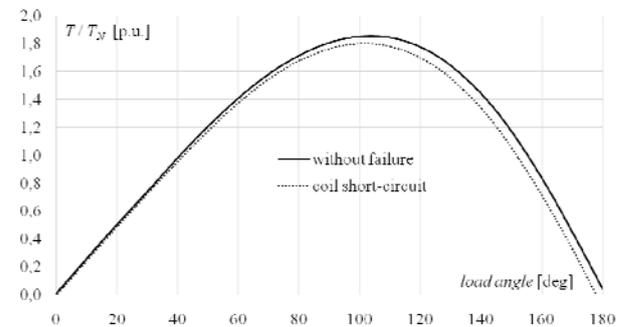
Fig. 9. Motor overload capacity in function of load angle
