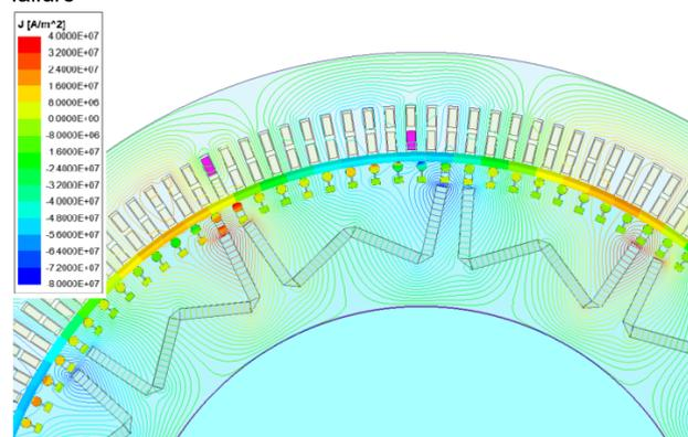
Fig. 14. Current densities in the rotor bars during rated load and with coil short-circuit
