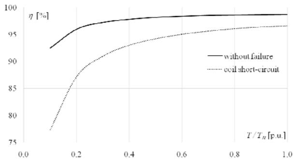
Fig. 10. Efficiency in function of load
