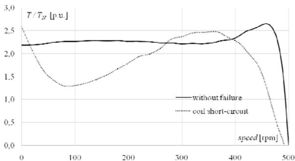
Fig. 15. Electromagnetic torque coming from the rotor cage
