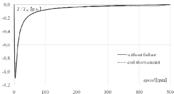
Fig. 16. Braking torque coming from the permanent magnet mounted in the rotor in function of speed
