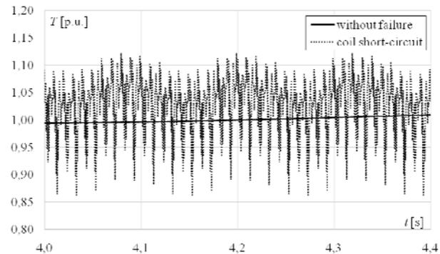
Fig. 8. Waveform of electromagnetic torque during rated load without failure and with coil short-circuit
