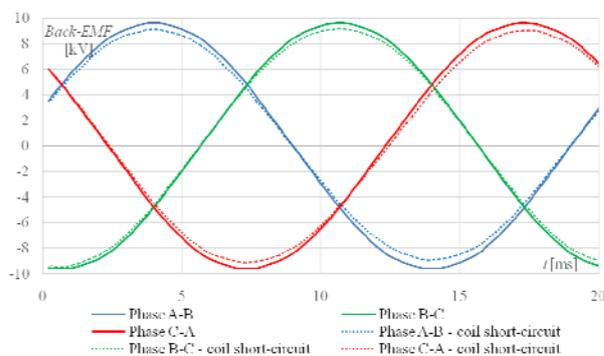
Fig. 3. View of electromotive forces induced on the stator terminals
