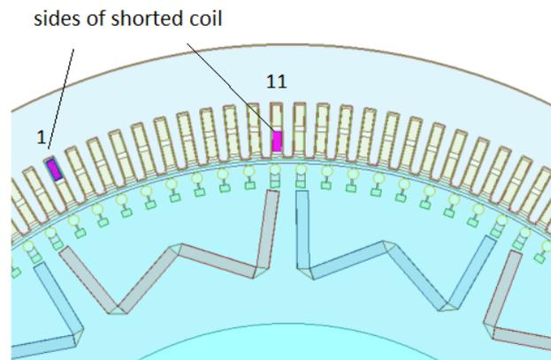
Fig. 2. View of coil short circuit in the stator winding of LSPMSM
