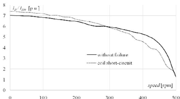
Fig. 17. Starting current in function of speed
