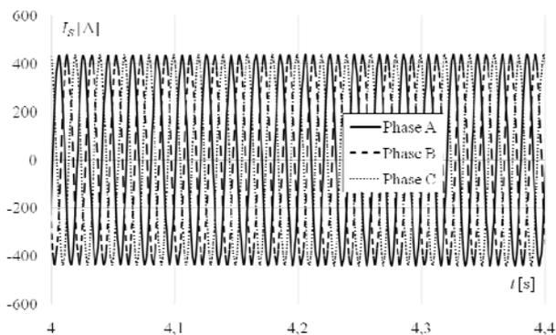
Fig. 6. Waveform of stator current during rated load (without failure)
