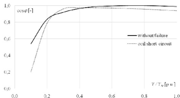
Fig. 12. Power factor in function of load
