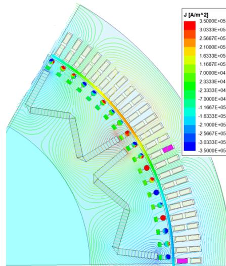
Fig. 13. Current densities in the rotor bars during rated load without failure
