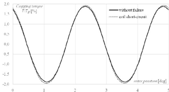
Fig. 5. Cogging torque in function of rotor position
