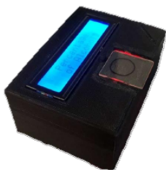
Fig. 2. Orthographic view of the fabricated alcohol sensor device
