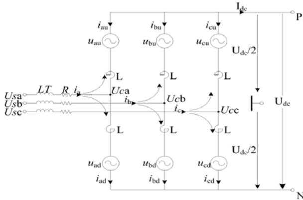
Fig.2. Equivalent circuit of MMC.
