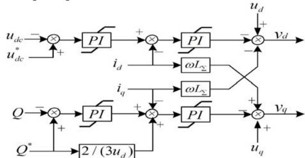
Fig.3. Block diagram of controller at Rectifier[17].
