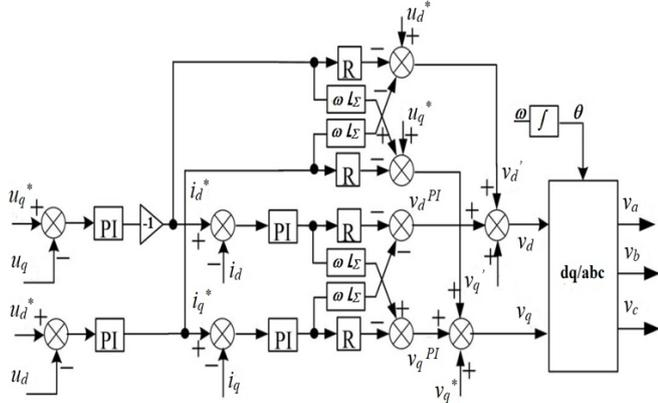
Fig.4. Block diagram of controller at inverter[17].
