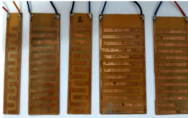
Fig. 3 Setup of Water Turbidity The fabricated the Interdigital Capacitor Sensor.
