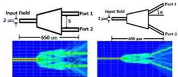
Fig. 5: The tapered design and the simulation result
