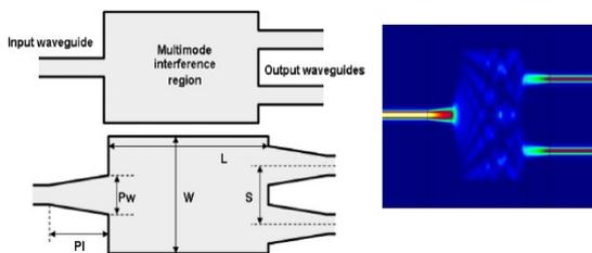
Fig. 4: The linear tapered of 1x2 MMI structure design [4]
