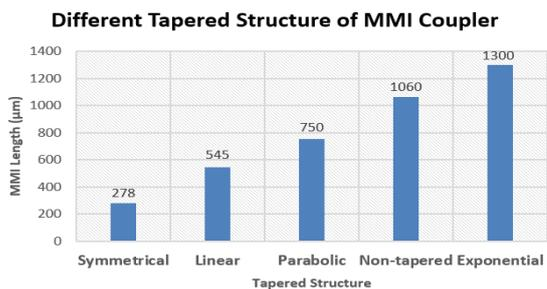
Figure 10: Length of different tapered MMI Couplers
