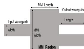
Fig. 2: The schematic diagram of the MMI splitter.
