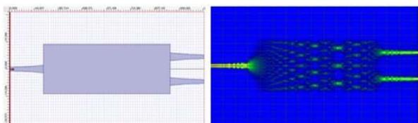
(c) Parabolic tapered MMI Coupler
