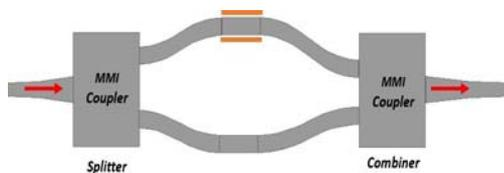
Fig/ 1: MMI Couplers in MZI optical modulator
