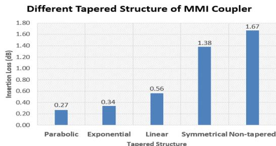
Fig. 9: Insertion Loss of different tapered MMI couplers
