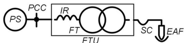
Fig.2. Conventional power supply scheme of EAF
