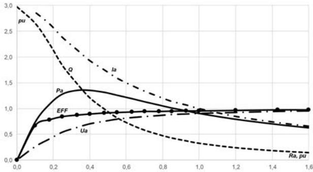
Fig. 5. The dependencies of indicators and parameters modes of EAF-3 furnace with CSC on the equivalent arc resistance
