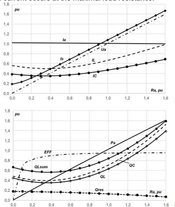
Fig.4. The indicators and parameters dependencies of EAF-3 mode with CC-CV converter on the equivalent arc resistance
