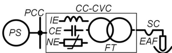
Fig.1. Structural diagram of EAF power supply with a non-valve CC-CV converter
