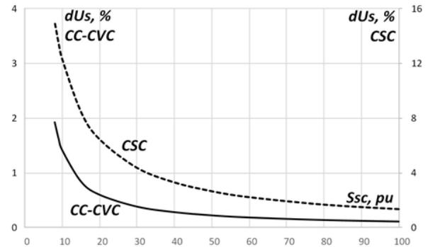
Fig. 6. The dependencies of the voltage changes in PCC on supply system power
