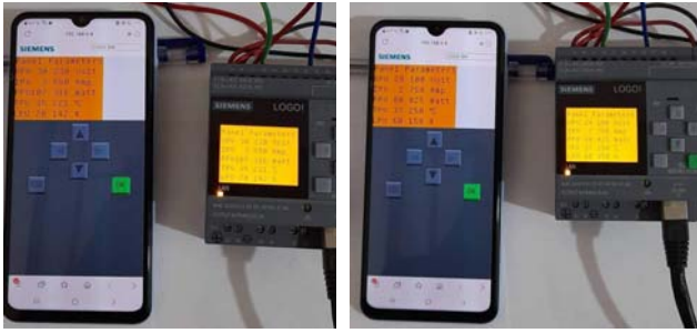
Fig. 6: Experimental Results: Message text on the PLC display unit, and smartphone.
