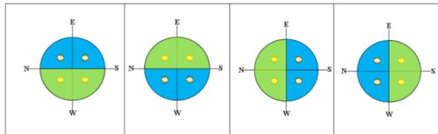
Fig. 4. Illustration of Two Sensors Exposed to the light, with Green as the exposed condition and Blue as the unexposed condition
