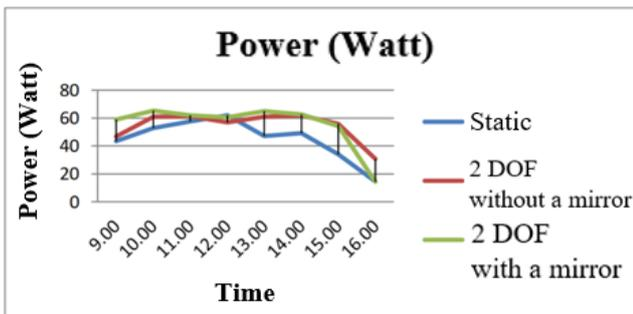
Fig. 7. Graph of PV Power against time in either static condition, 2 DOF without a mirror, and 2 DOF with a mirror
