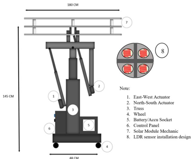
Fig. 2. Mechanical System Design
