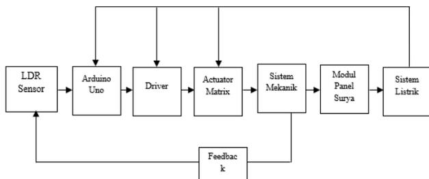
Fig. 1. Photovoltaic Panel Position Control System Design
