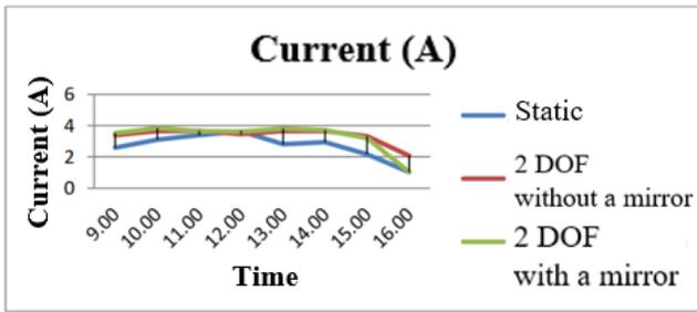
Fig. 6. Graph of PV Current against time in either static condition, 2 DOF without a mirror, and 2 DOF with a mirror
