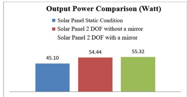
Fig. 8. Comparison Graph of Overall Output Power Average of Solar Panel
