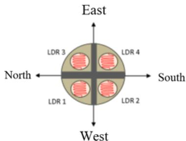
Fig. 3. LDR Sensor Position Installation
