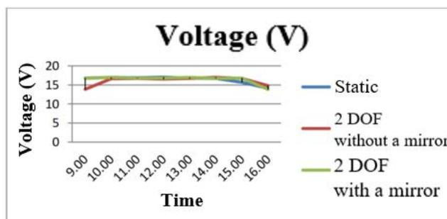
Fig. 5. Graph of PV Voltage against time in either static condition, 2 DOF without a mirror, and 2 DOF with a mirror
