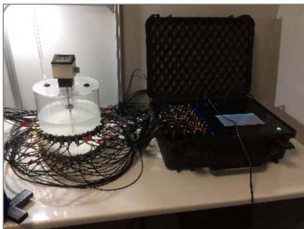
Fig. 3. The test stand: on the left side is the reactor model with electrodes, and on the right side there is a tomograph
