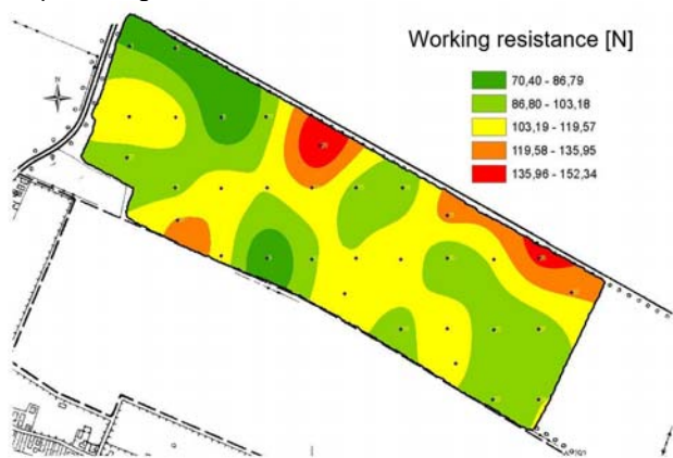
Fig. 5. Spatial variation of the resistance force of the drill coulters at the depth of potential seed sowing
