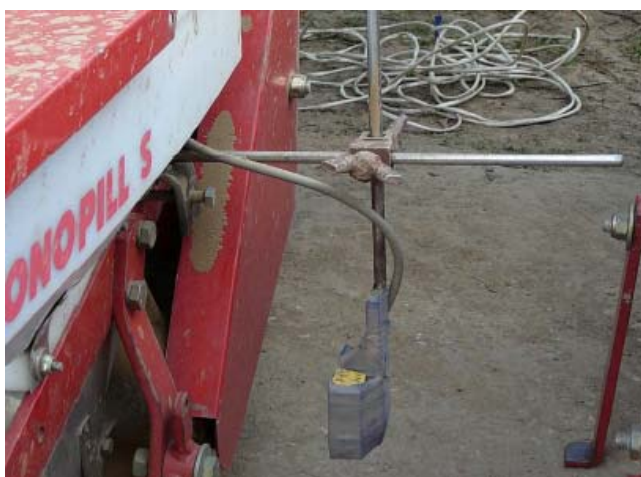
Fi. 2. Location of the optical distance sensor
