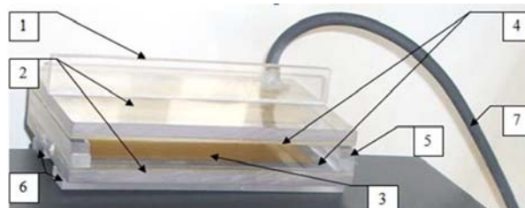
Fig.1. Test bench components: 1 – handgrip, 2 – plates (external and internal), 3 – brass plate, 4 – capacitor plates (electrodes), 5 – distance plate, 6 – supports, 7 – cable connecting the top and bottom capacitor plates with the power supply system [28]
