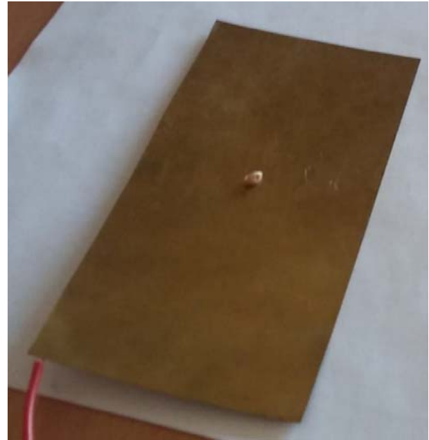
Fig.5. Brass plate for removing electric charge during measurements [28]
