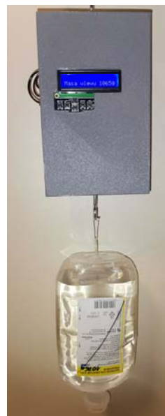
Fig. 4. The developed concept of the infusion fluid level monitoring system.
