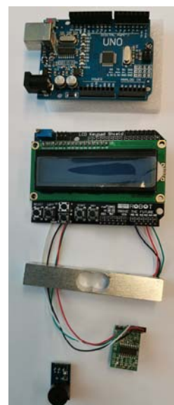
Fig. 2. Electronic components of the scale (from the top: Arduino UNO board, LCD Keypad Shield, strain gauge with signal conditioning and tensometric beam; buzzer in the left lower corner).
