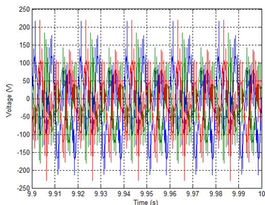
Fig.19. Injected voltage of three-level series active filter
