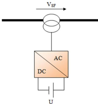
Fig.3. Series active power filter
