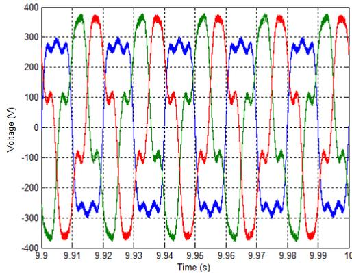
Fig.12. Network disrupted voltage
