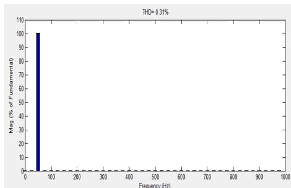
Fig.21. Voltage spectral analysis
