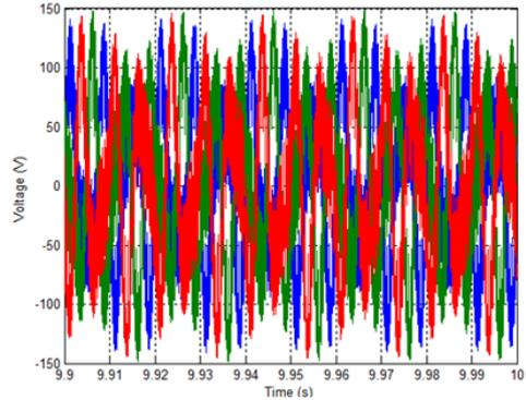
Fig.14. Series active filter voltage
