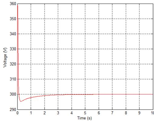
Fig.11. DC link of inverter
