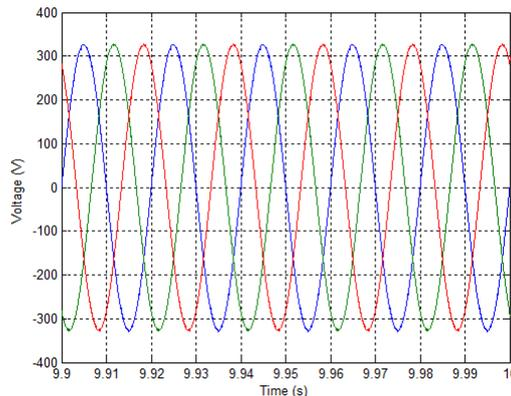
Fig.20. AC micro-grid voltage
