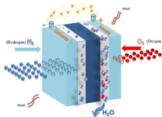
Fig.1. Schematic of PEM fuel cell operation
