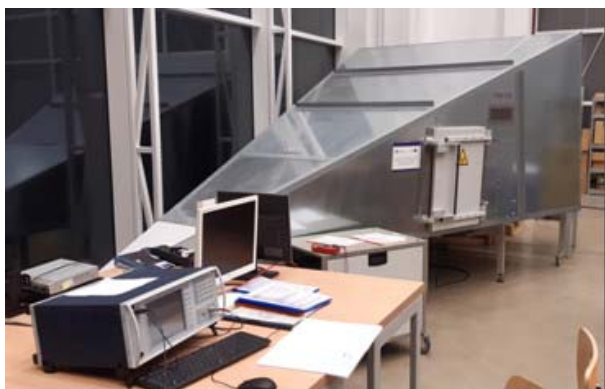
Fig. 1. Radiated disturbance test stand
