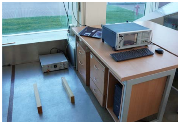
Fig. 2. Transmitted disturbance test stand
