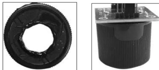
Fig. 4. Setup of tip area for TCS3200
