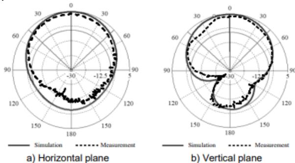
Fig. 11. 2D Radiation pattern for the trapezoidal patch with a multi-slot antenna from simulation and measurement
