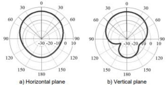
Fig. 8 2D radiation pattern from simulation of the trapezoidal patch with a multi-slot antenna
