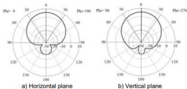
Fig. 3. 2D radiation pattern from the simulation result of the rectangular patch antenna
