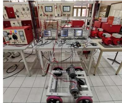
Fig.7. Experimental Test-rig for the dual motor belt drive in the laboratory study.
