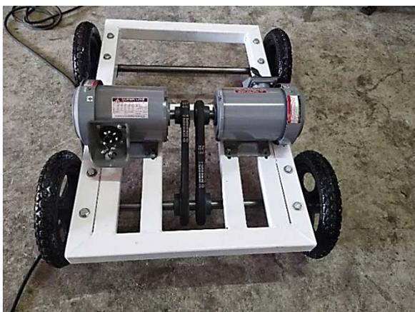
Fig.3. Photograph of the proposed simplified dual motor belt drive model.
