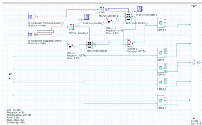
Fig.11(a). 100Gbit/s WDM system transmitted component with ROADM architecture in 200Km length FO
