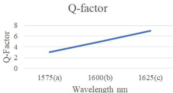
Fig.13. Effects wave length on transmission qualité for 200Km
