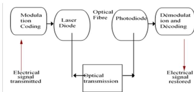
Fig.4. Optical fiber transmission chain
