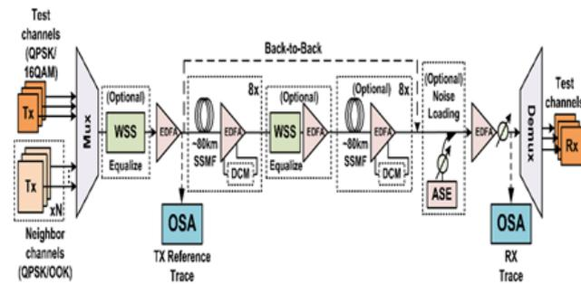
Fig.5. Schematic of experimental fiber transmission link
