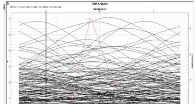
Fig.9 (b). Eye diagram for 100Gbit/s transmission with 50km length FO
