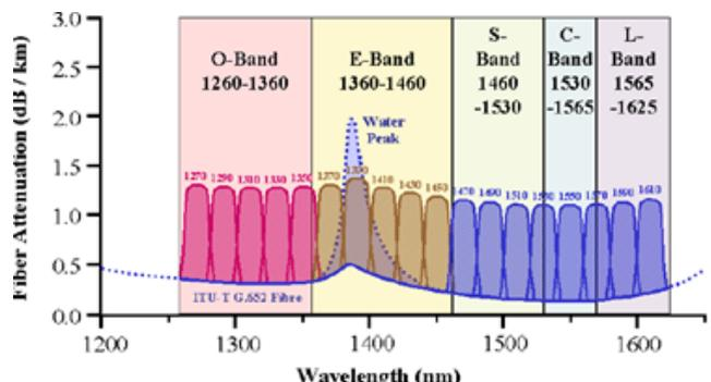
Fig.3. CWDM and DWDM frequency Band
