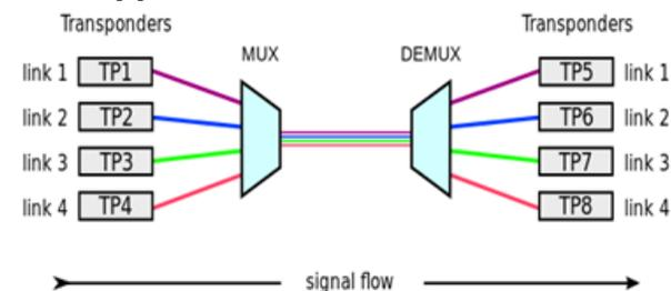
Fig.1. Schematic of a WDM system
