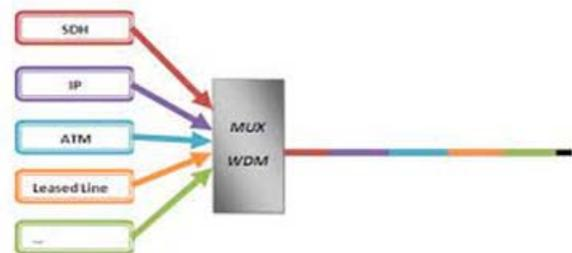
Fig.2. Principe Multiplexing with different protocols
