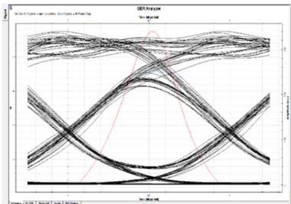
Fig.10(b). Eye diagram for 100Gbit/s transmission with 100Gbit/s
