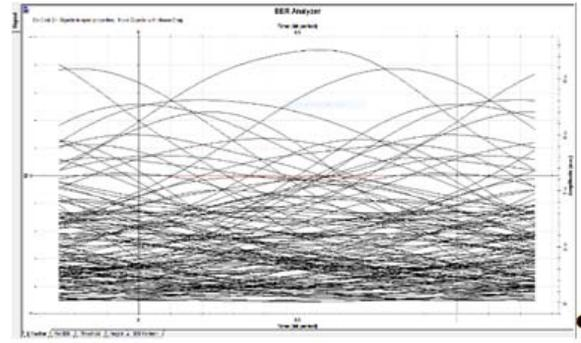
Fig.9 (a). Eye diagram for 100Gbit/s transmission with 40km length FO
