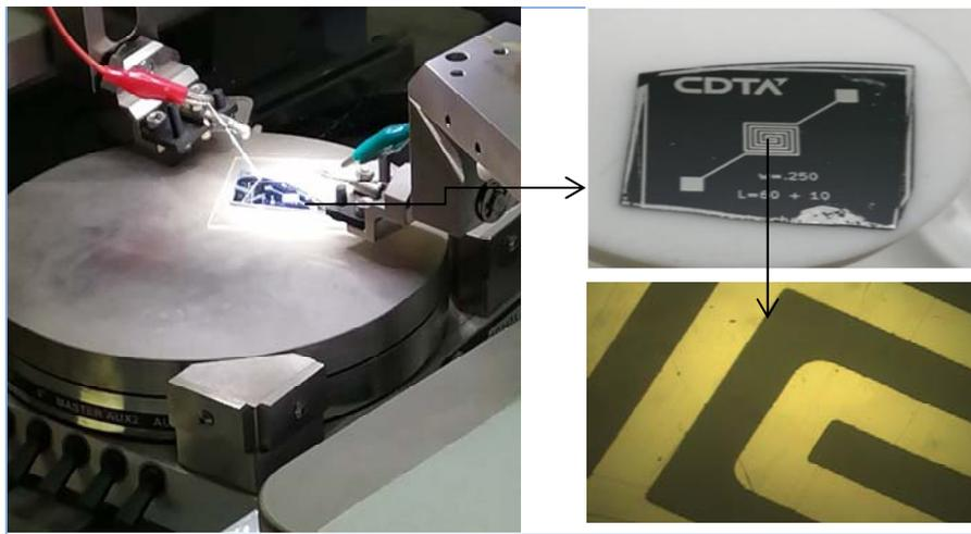
Fig.3. Presentation of the realized experimental model of the sensor
