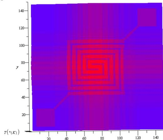
Fig.8. The temperature distributions simulated by TLM method for micro-heater
