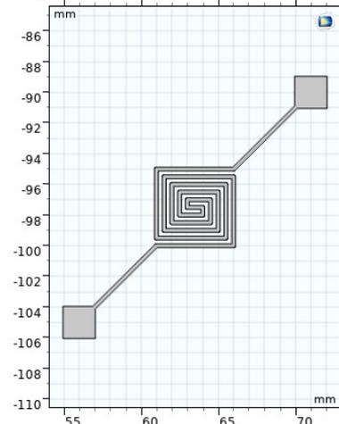
Fig.2. Micro-hotplate structure with a platinum heater
